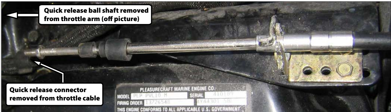
Step 2 Side/Top Engine View Remove the quick release connector from existing throttle cable. Remove quick release ball from throttle arm.
