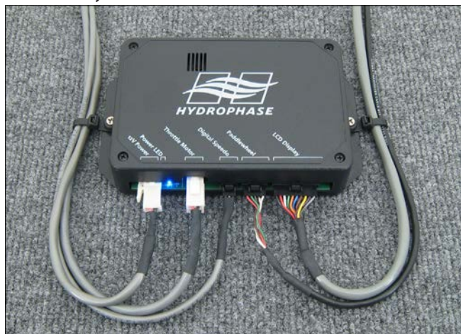
Figure 12-1: CPU mounted to an inside wall under the dash. Alternatively, the included zip ties may be used to secure it to other convenient under-dash locations.
