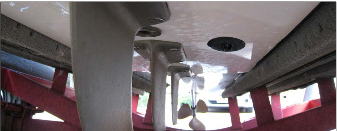
Figure 16-3: 1992 Malibu Sunsetter Inboard : [view from bow / front of boat] Paddlewheel located slightly back from drain plug and about 6" from centerline. Locate paddlewheel as far back as possible while maintaining obstruction-free path in front of paddlewheel.
