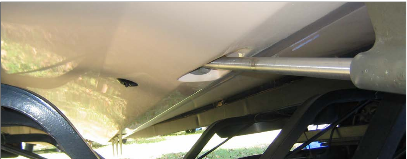
Figure 16-2: 2001 Ski Nautique V-drive : [view from stern / rear of boat] Paddlewheel located about 56" from stern (rear end) and about 7" from centerline.
