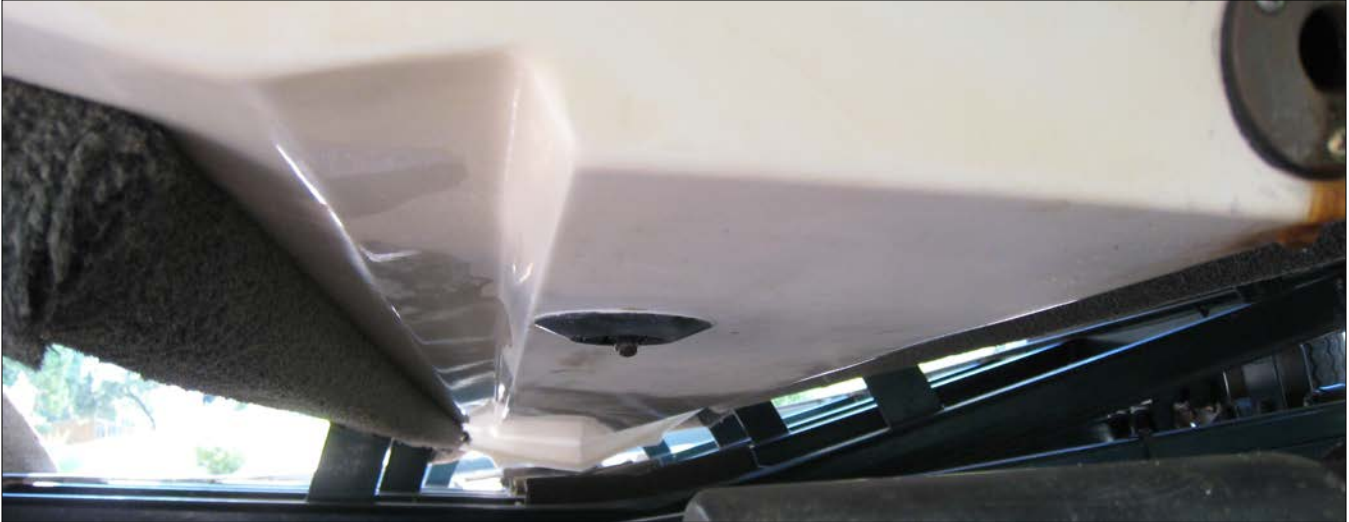
Figure 16-1: 2000 Regal 2100 LSR I/O : [view from stern / rear of boat] Paddlewheel located about 8" from stern (rear end) and about 5" from centerline.
