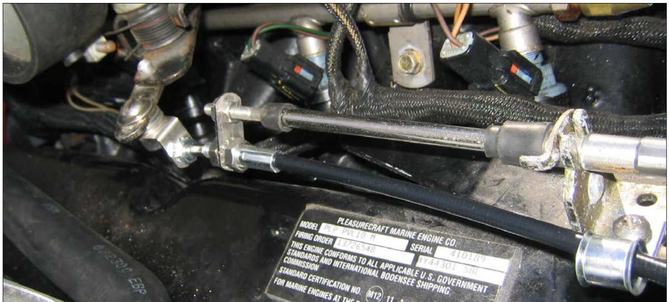
Step 9 Finished control cable installation should look similar to the picture above. The control cable should be approximately parallel to the existing throttle cable from the cable guide to the throttle arm. To align, loosen throttle / control cable nuts, align cable, then re-tighten nuts. Replace the spark arrestor and/or engine cover if previously removed. Make sure control cable continues to be clear of any obstructions. NOTE: The driver throttle lever is in the wide open (full down) position for photo purposes.
