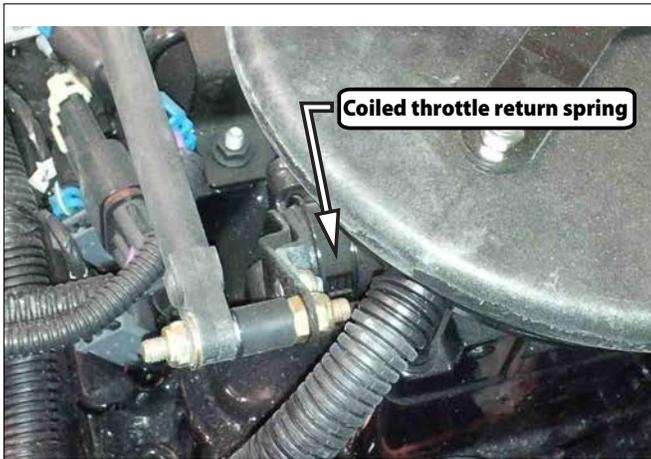
Figure 12-2: Coiled throttle return spring on Mercruiser 4.3L MPI engine
