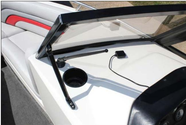
Figure 15-1: GPS receiver mounted on the dash beneath the windshield.
