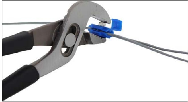
**4.** Make sure the two wires are centered properly in the connector. Use pliers to push the blade into the connector. This will pierce the insulation of the two wires and electrically connect them. It will also securely hold them together.
