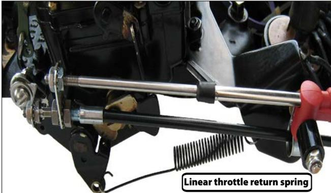
Figure 12-1: Linear throttle return spring on Mercruiser 5.7L engine
