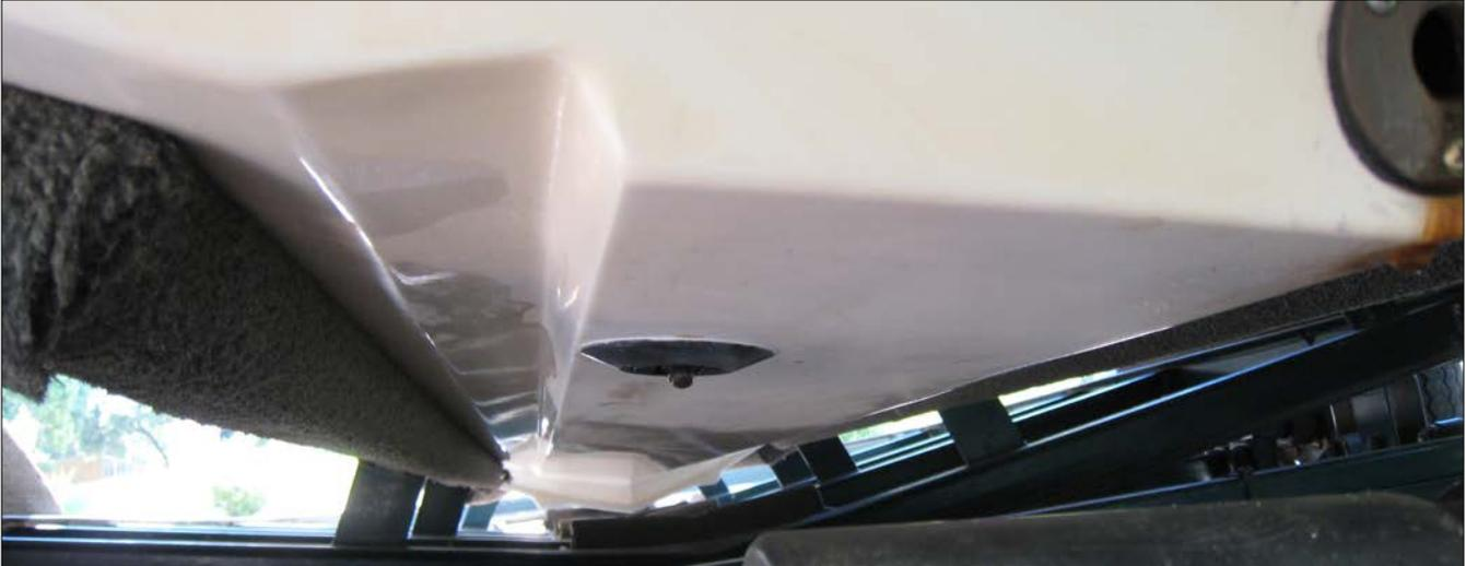
Figure 20-1: 2000 Regal 2100 LSR I/O: [view from stern / rear of boat] Paddlewheel located about 8" from stern (rear end) and about 5" from centerline.
