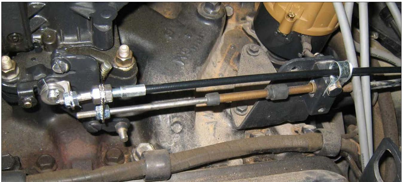
**Step 9** Finished control cable installation should look similar to the picture above. The control cable should be approximately parallel to the existing throttle cable from the cable guide to the throttle arm. To align, loosen throttle / control cable nuts, align cable, then re-tighten nuts. Replace the spark arrestor and/or engine cover if previously removed. Make sure control cable continues to be clear of any obstructions.
