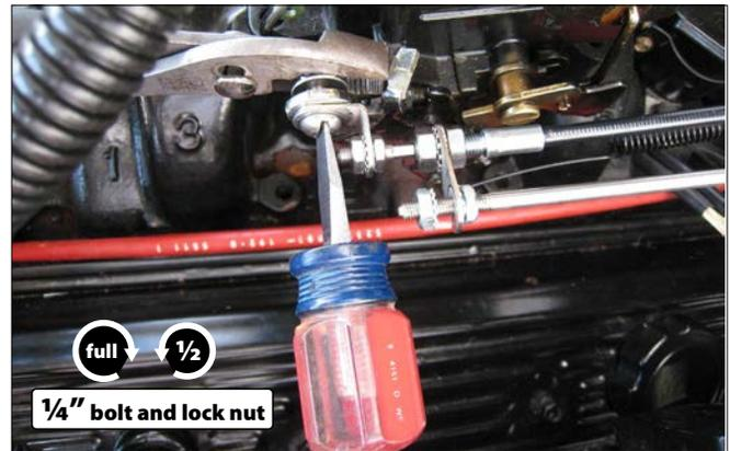
**Step 6** Tighten the 1/4" slotted bolt and nylon lock nut fully with screwdriver and pliers then un-tighten 1/2 turn. L-bracket should be snug but able to swivel freely on the throttle arm.
