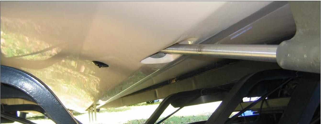
Figure 20-2: 2001 Ski Nautique V-drive: [view from stern / rear of boat] Paddlewheel located about 56" from stern (rear end) and about 7" from centerline.
