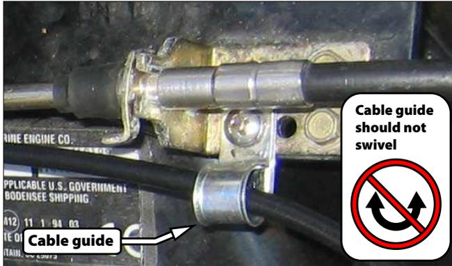
**Step 5** Install cable guide onto existing throttle cable bracket as shown using the 10-32 x 1/2" bolt and nylon lock nut provided. Tighten with pliers and screwdriver enough that the cable guide will not move as the cable passes through it.
