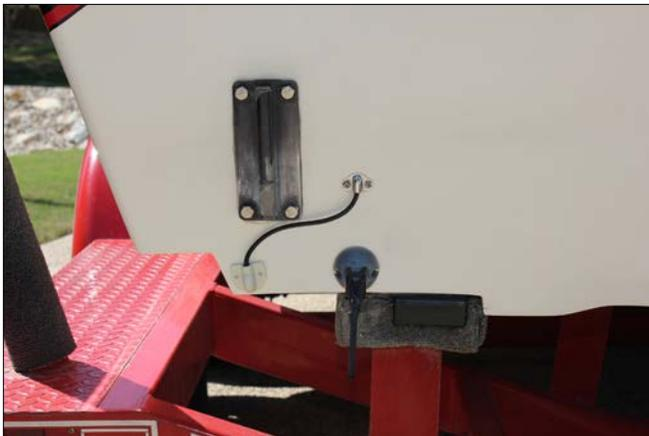
Figure 15-2: Water temperature sensor mounted on transom using existing pitot tube hole
