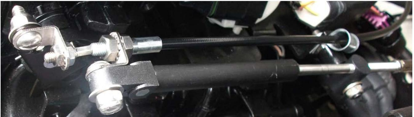
Figure 31-4: [side/top view] Horizontal orientation with existing throttle cable moved back. This is the preferred method for installing on many Mercruiser I/Os. It can also be fitted vertically for engines without the long throttle cable mounting point bolts and spacer.
