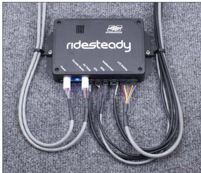
Figure 16-1: CPU mounted to an inside wall under the dash. Alternatively, the included zip ties may be used to secure it to other convenient under-dash locations. Note the throttle motor power cable is only "bundled" with the power cable.
