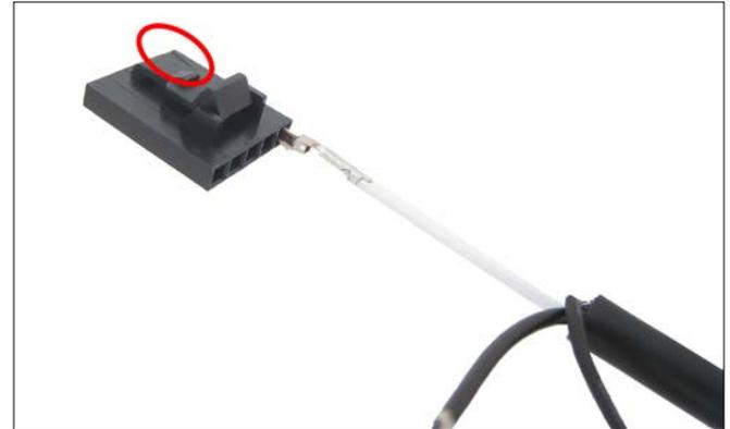
Figure 15-3: Position the white wire just inside the slot on right, denoted by the small arrow (in circle above). The small “retention clip” of the contact should be oriented downwards.
