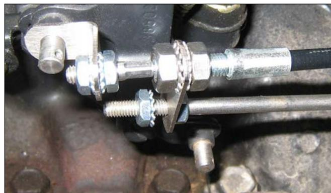
**Step 4** Install the control cable onto the existing throttle cable using two K-lock nuts as shown. Place the L-bracket onto the throttle arm shaft as shown. **NOTE:** Moving the driver throttle lever about half way down may help with clearance.
