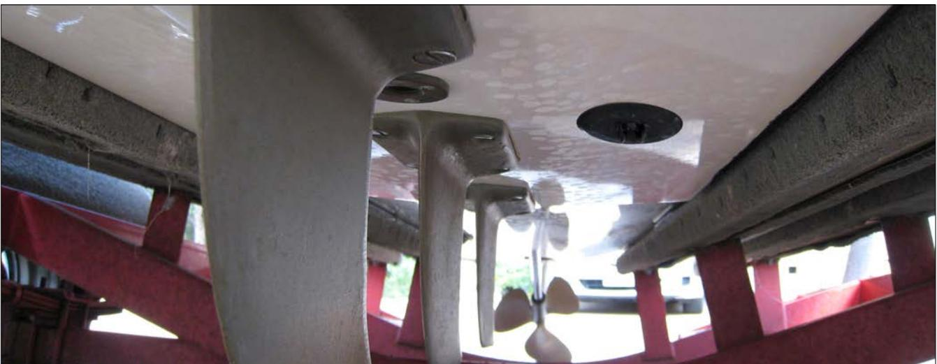
Figure 20-3: 1992 Malibu Sunsetter Inboard: [view from bow / front of boat] Paddlewheel located slightly back from drain plug and about 6" from centerline. Locate paddlewheel as far back as possible while maintaining obstruction-free path in front of paddlewheel.
